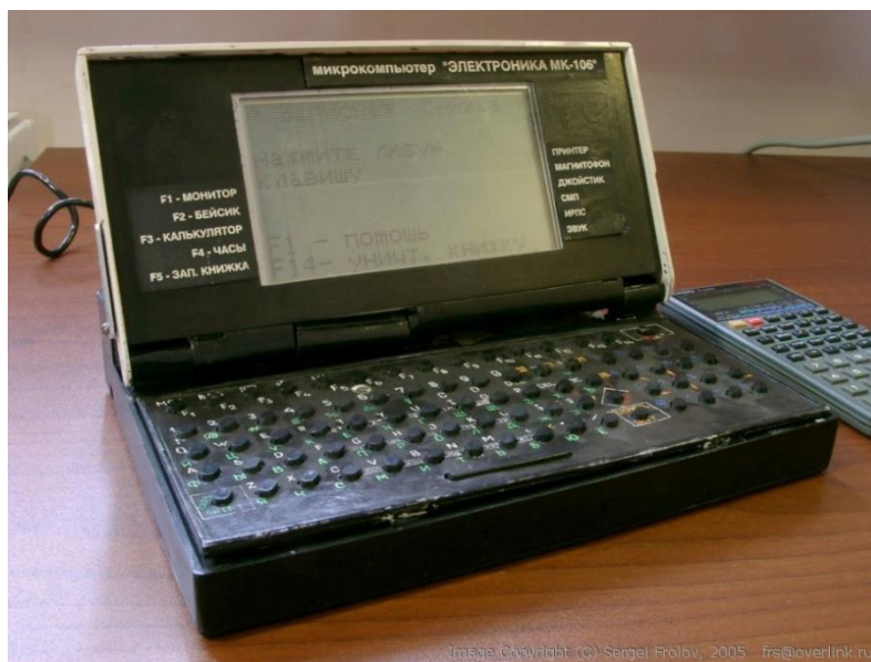
Figure 6. Soviet laptop –“Electronica MK-106” (with the letter ё)
