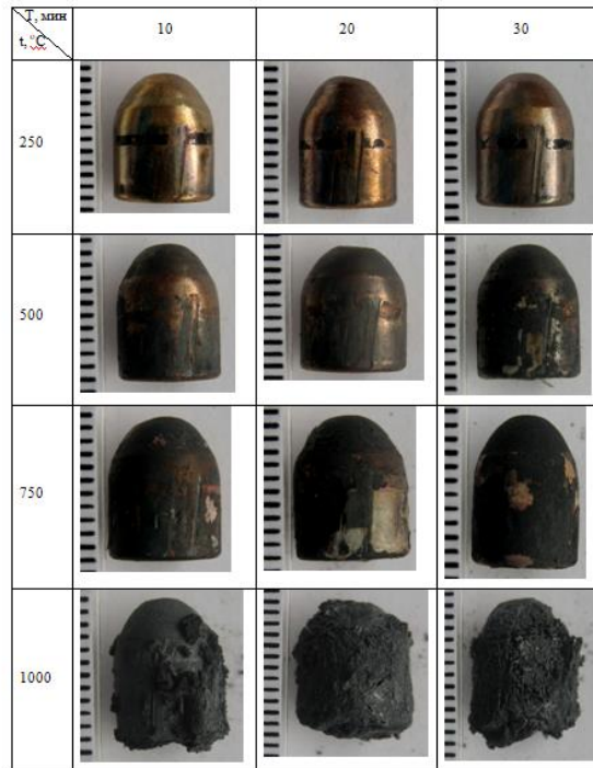
Figure 2. Changes recorded in bullets fired from a 9 mm Makarov pistol that were subjected to high temperatures (temperature – 250, 500, 750 and 10000 °C, exposure time to heat – 10, 20 and 30 min.)
